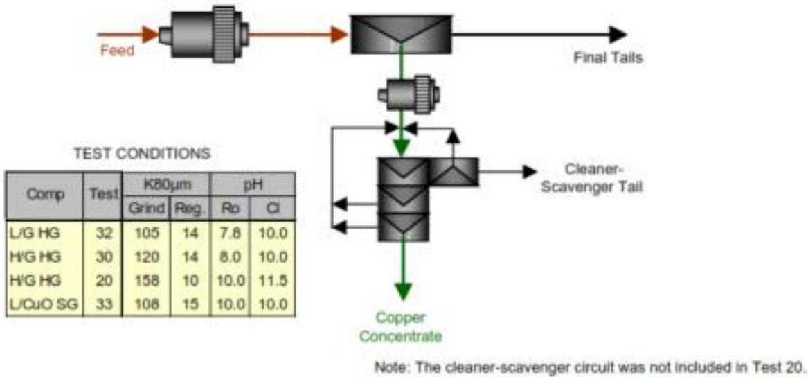
**CYCLE TEST METALLURGICAL BALANCE DATA**
