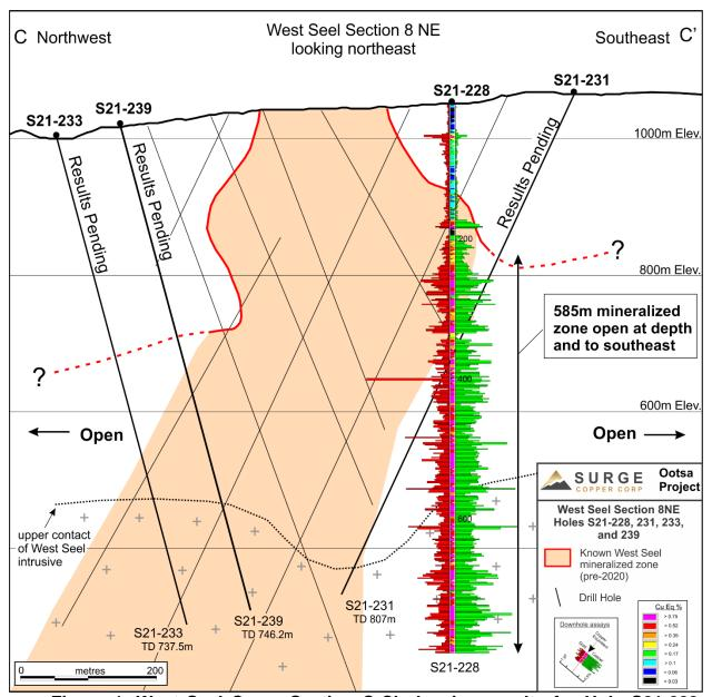
Figure 1. West Seel Cross Section C-C' showing results for Hole S21-228. See Figure 2 for section location.
