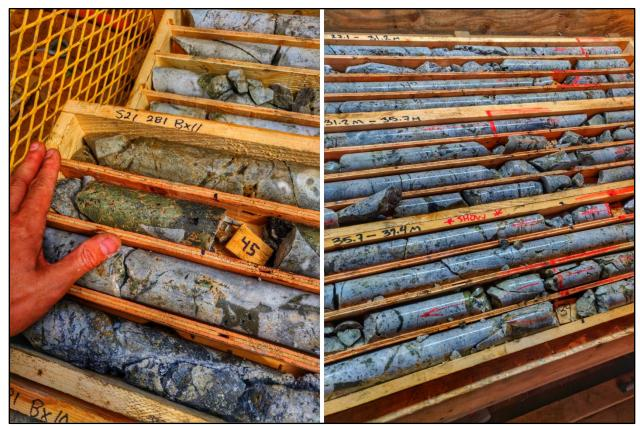
Figure 3. Photographs from recent drilling at the Seel Breccia Zone. Left: 20-centimetre-wide semi-massive chalcopyrite zone within a widespread breccia from 45 metres depth in hole S21-281. Right: Breccia zone from 27 to 37 metres in hole S21-270. Note large blebs of chalcopyrite throughout the breccia matrix.
