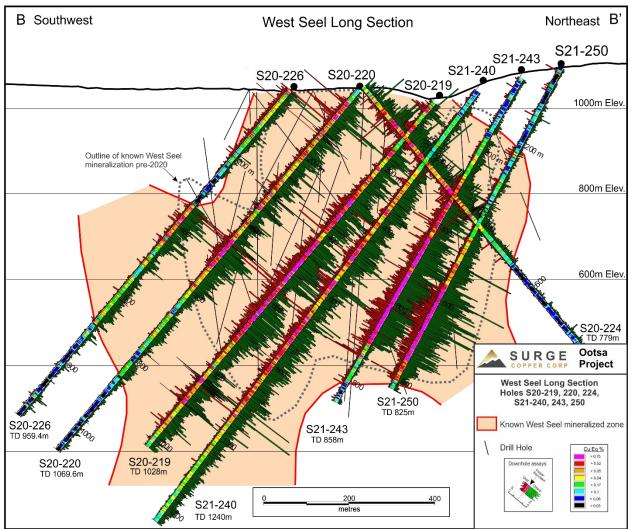
Figure 2. West Seel long section B-B' showing results for holes S21-219, 220, 224, 226, S21-240, 243, and 250. See Figure 1 for section location.
